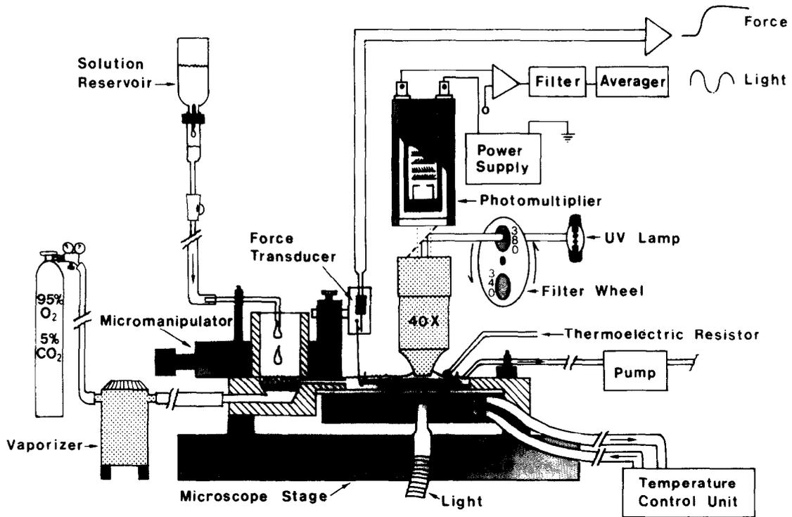
Fig. 1 Schematic diagram of the experimental set-up used to record fluorescence from the human skeletal muscle fibers
